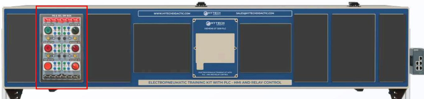
The Push Button and Selector Switch Module serves as a key manual input interface for relay-based operations in the Hytech Electrohydraulic Training Kit. It features industrial-grade push buttons and selector switches that let users manually initiate, interrupt, or toggle control signals during experiments.
