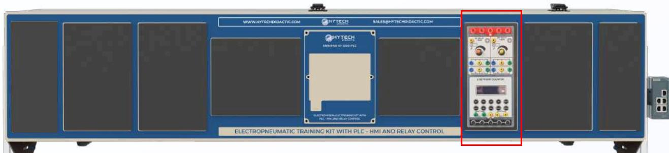
The Electronic Timer and Counter Module enhances relay-based operations in the Hytech Electrohydraulic Training Kit by adding time-delay and event-counting functions. It enables users to implement dynamic control logic such as delayed actuator movement and cycle counting.
