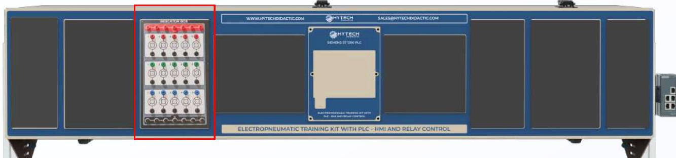
The Indicator Module enhances the Hytech Electrohydraulic Training Kit by providing real-time visual feedback during relay-based experiments. With 15 LED indicators, it allows users to monitor the status of signals and outputs within a control circuit.
