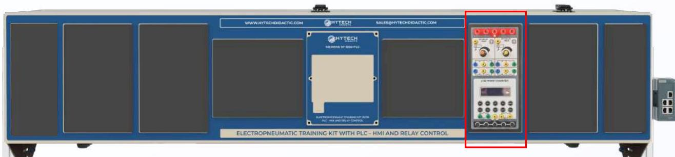
The Electronic Timer and Counter Module enhances relay-based operations in the Hytech Electropneumatic Training Kit by adding time-delay and event-counting functions. It enables users to implement dynamic control logic such as delayed actuator movement and cycle counting.
