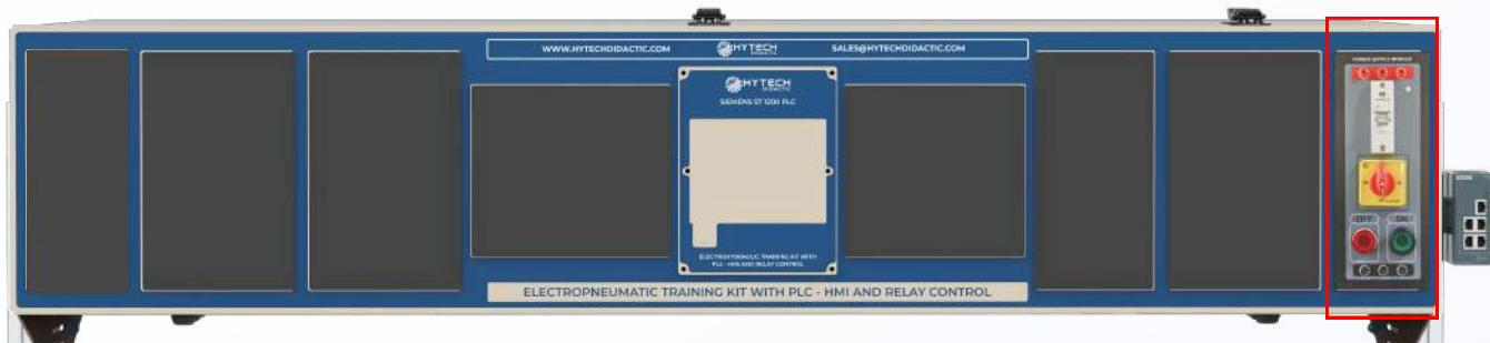
The Power Bank and Power ON Module is a key component of the Hytech Electropneumatic Training Kit, providing centralized control and safe power distribution across the entire system. It simplifies operation, enhances safety, and ensures consistent performance of all training modules.
