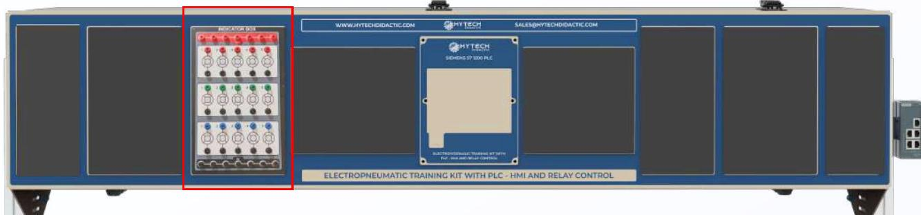
The Indicator Module enhances the Hytech Electropneumatic Training Kit by providing real-time visual feedback during relay-based experiments. With 15 LED indicators, it allows users to monitor the status of signals and outputs within a control circuit. This module improves functionality, supports faster troubleshooting, and helps students better understand circuit behavior—making it an essential tool for developing core automation skills.
