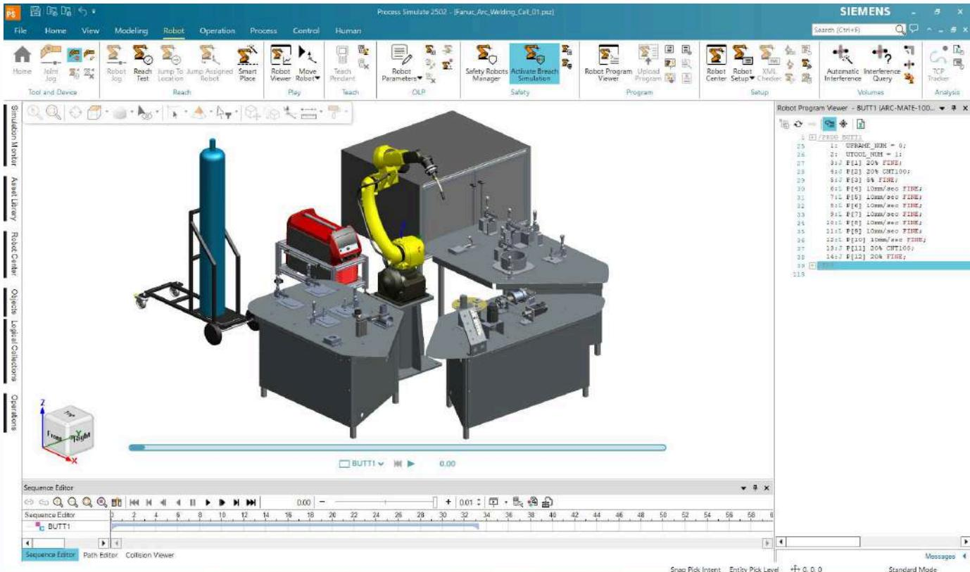
In modern technical education, robotic welding training cells are no longer just physical setups — they are platforms to teach smart manufacturing, automation, and Industry 4.0 concepts. Two critical components that elevate the effectiveness of these cells are Digital Twin and Offline Programming.
