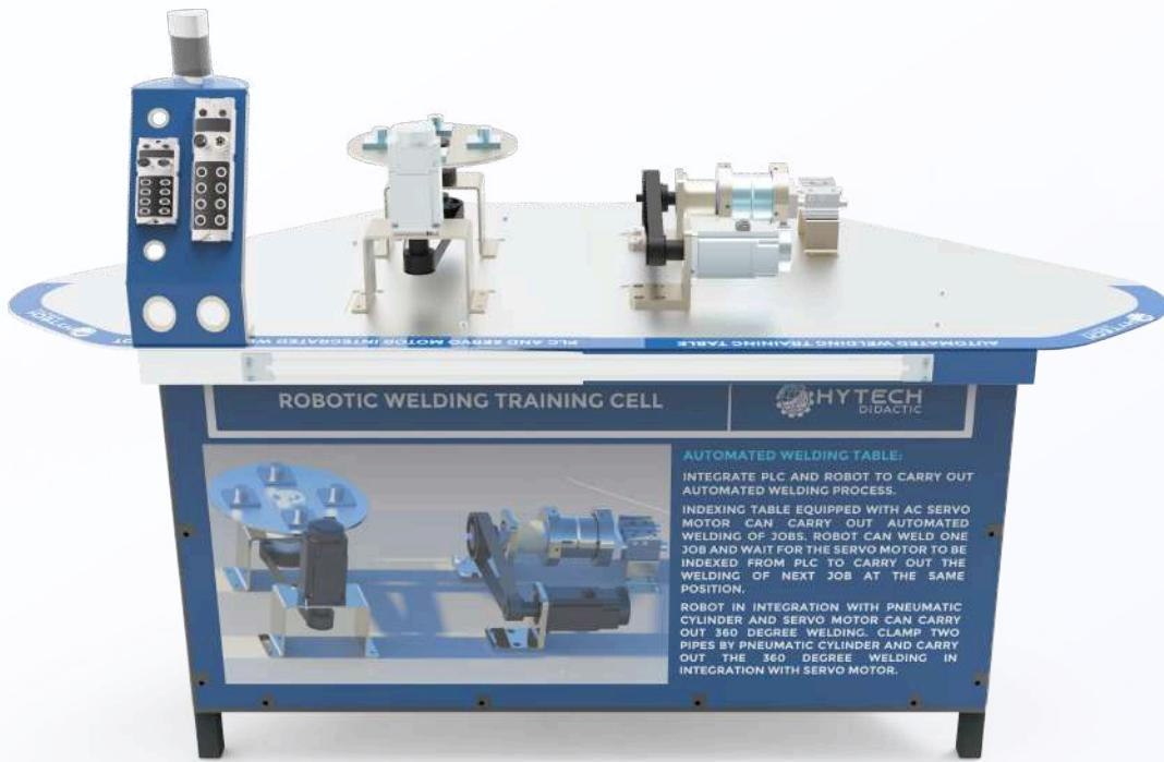
The Automated Welding Table is equipped with integrated fixtures, sensors, and sometimes motion systems to support fully automated welding operations. It allows the robot to work with minimal human intervention, increasing productivity and repeatability. This table is typically used for batch production or complex welding cycles where automation maximizes efficiency and consistency.
