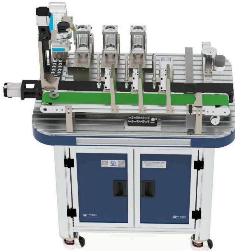
Station 1 is equipped with a pneumatic gauging system that sorts three different types of bearings with the same outer diameter but varying inner diameters. Any bearing other than the three predefined types will be rejected at Station 1.
