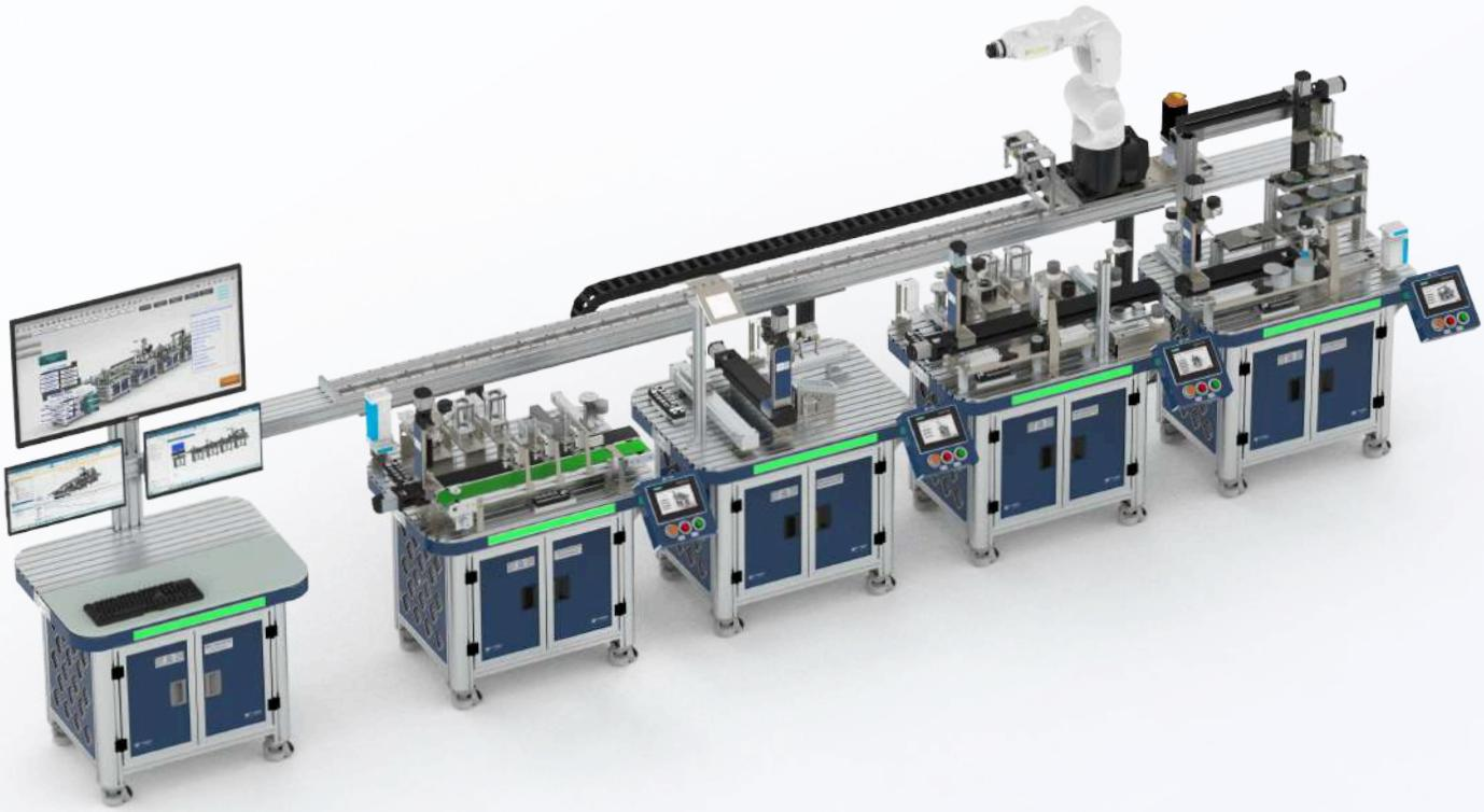
Smart Factory is a robotic setup with connected machines. It can also be called as a Modular Production System (MPS) with IIOT Integration.
