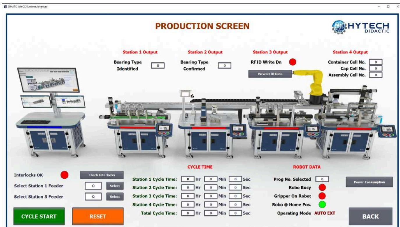
The **SCADA (Supervisory Control and Data Acquisition)** system is a powerful integration of **hardware and software components** that enables **real-time supervision, control, and data acquisition** across the entire automation environment. SCADA ensures seamless interaction between operators and field-level devices, both **locally and remotely**, via a centralized control interface.
