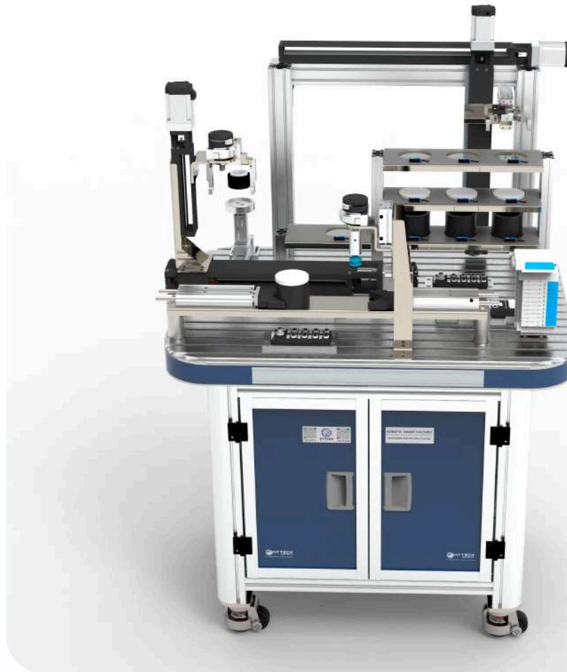
The ASRS Cartesian robot retrieves a container and cap from the ASRS storage rack. The servo motor-based rotary pick-and-place module picks up the container and cap from the ASRS storage rack and transfers them to the Capping Module. In the Capping Module, the container cap is securely fixed onto the container using a vacuum-based suction mechanism. After capping, the system transfers the capped container back to the ASRS storage rack.
